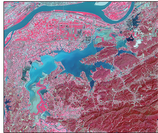
Fig.2 Sentinel-2 acquired the 23/03/2018. False color composite, with B8, B4 and B3 in RGB (tiles 50RMU and 50RNU)
